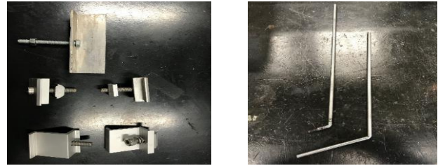
Fig. 6: Connectors used for fixing the modules - Fig. 7: Small rods used in the tests
