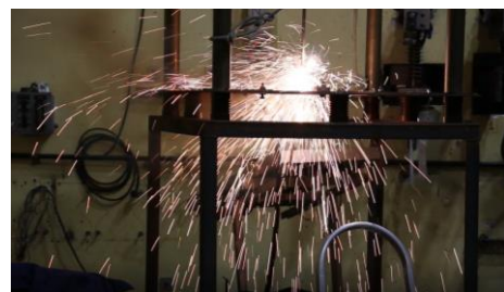
Figure 8: Arc in gap during the test
